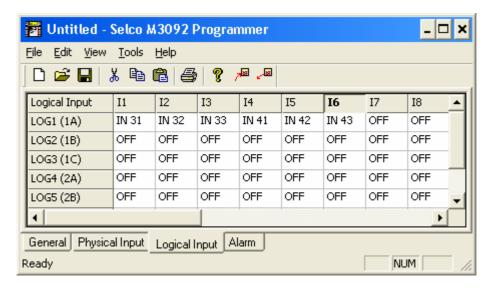
Each of 12 input references can point to any physical or logical input. Input references that are not required must be set to "OFF". In the example above LOG1 will be calculated as the average of IN31, IN32, IN33, IN41, IN42 and IN43.
